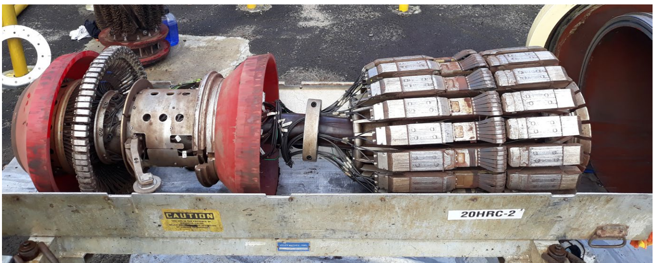
Figure 5.8 A magnetic flux leakage inline inspection tool known as a pig
