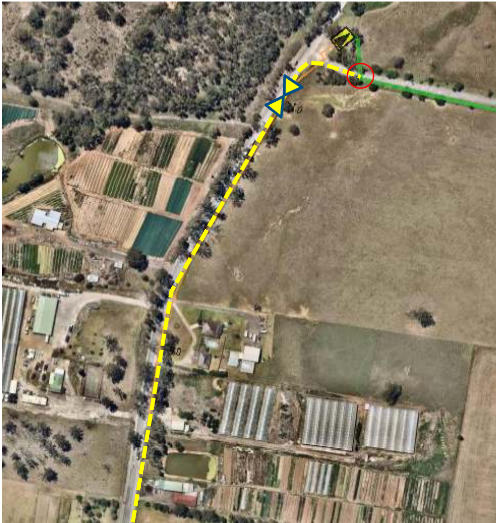
Secondary mains continue along Badgerys Creek Road and tie into secondary mains
