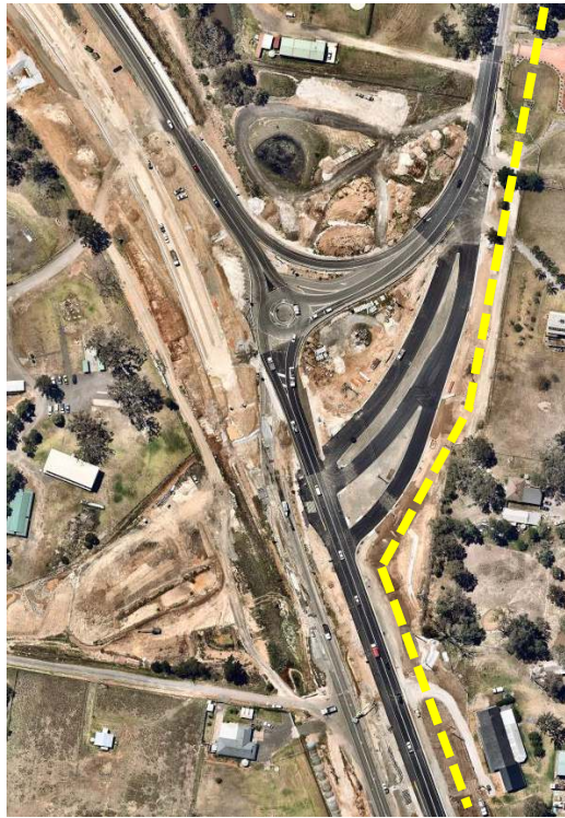
The secondary main is proposed to continue along The Northern Road before going up Badgerys Creek Road
