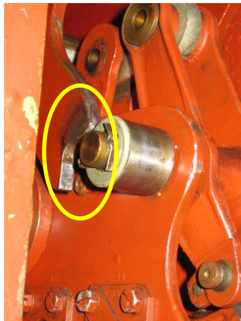
Photo 2: Worn Hold on Catch
