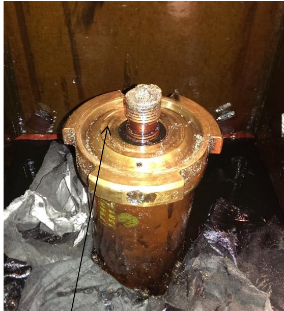
Picture 2: The white phase fixed contact cluster is removed from the shaft. The heat generated from the contact failure caused 2 threads to melt away. Local judgement ascertained that the current carrying capability is not through the thread but primarily through the base of the contact as indicated by the arrow. Therefore the old thread was retained and new contacts were installed.
