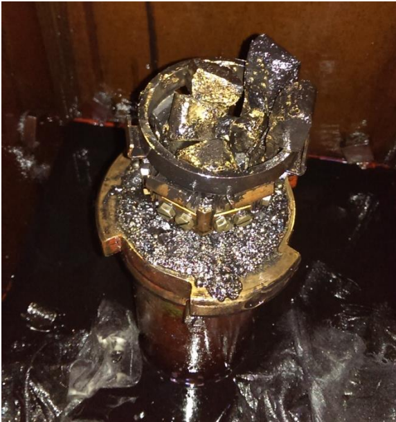
Picture 1: The 22kV white phase fixed contact suffered significant damage. Due to the extent of the damage it is difficult to ascertain the cause but it is anticipated that a small spring that sits behind a contact finger has lost compression and created a high resistance connection.
