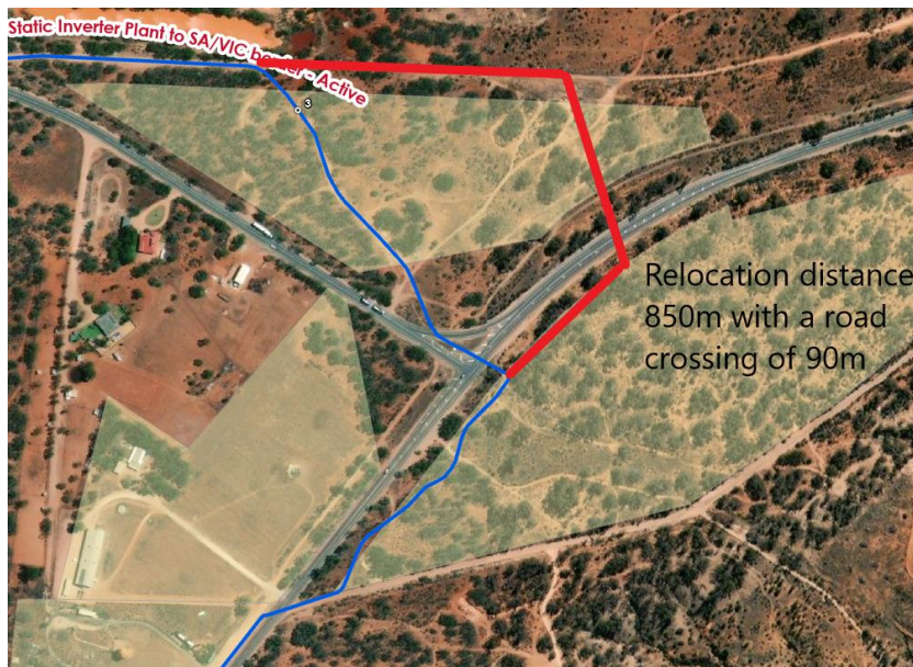
Murraylink cable (blue line) and proposed relocation (red line) to avoid future Sturt Highway intersection upgrade.
