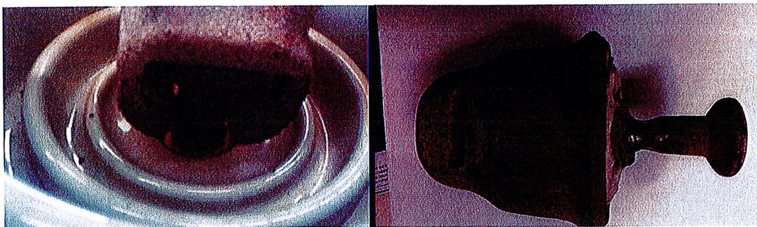
Figure 2 - Example Corrosion and section loss after cleaning on 132kV Insulator Disc from Tower 9A
