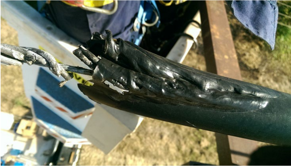
Figure 5 Damaged conductor Due to “poly-pipe” bat guards
