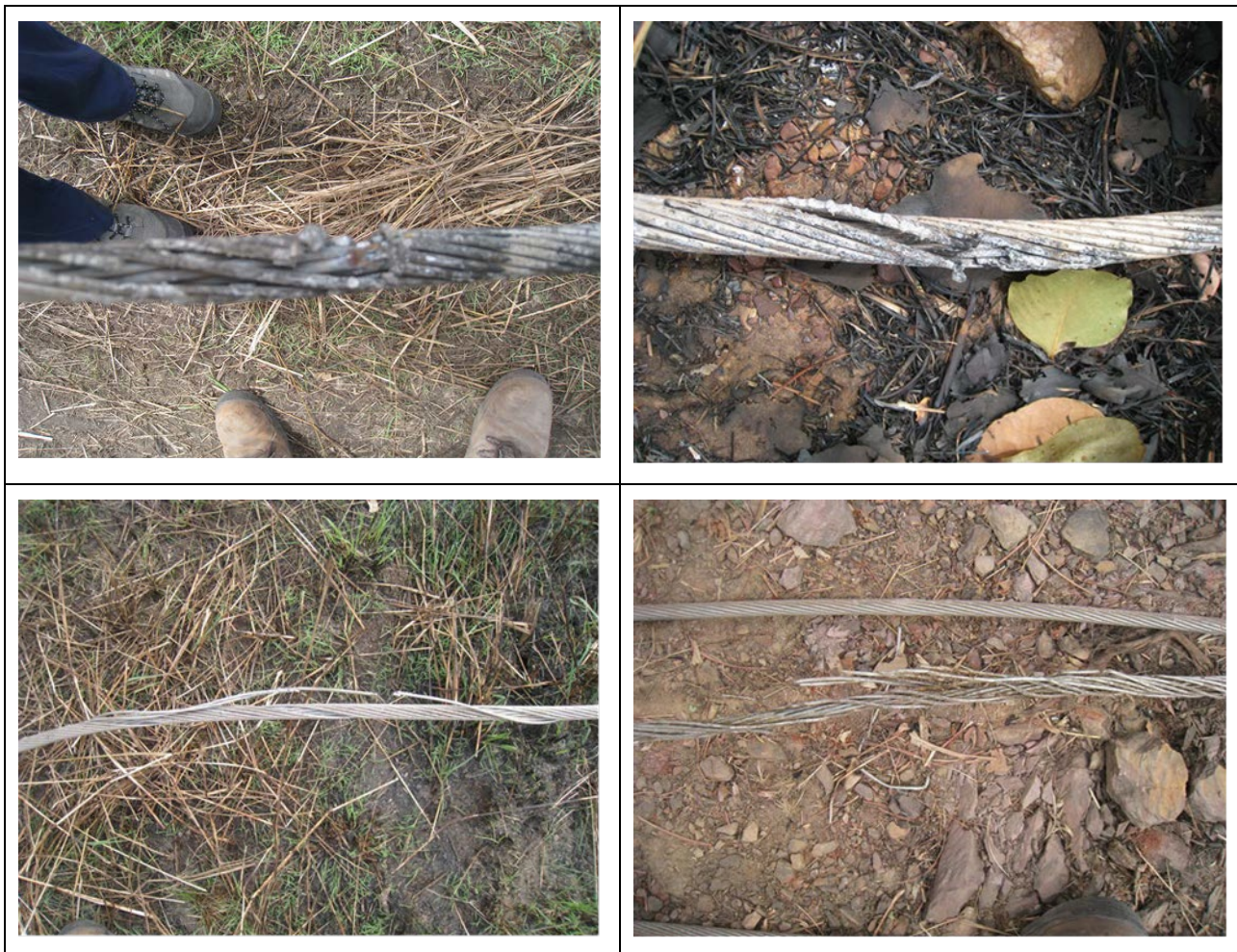
Figure 4 Cockatoo conductor photos showing broken strands, burning and corrosion
