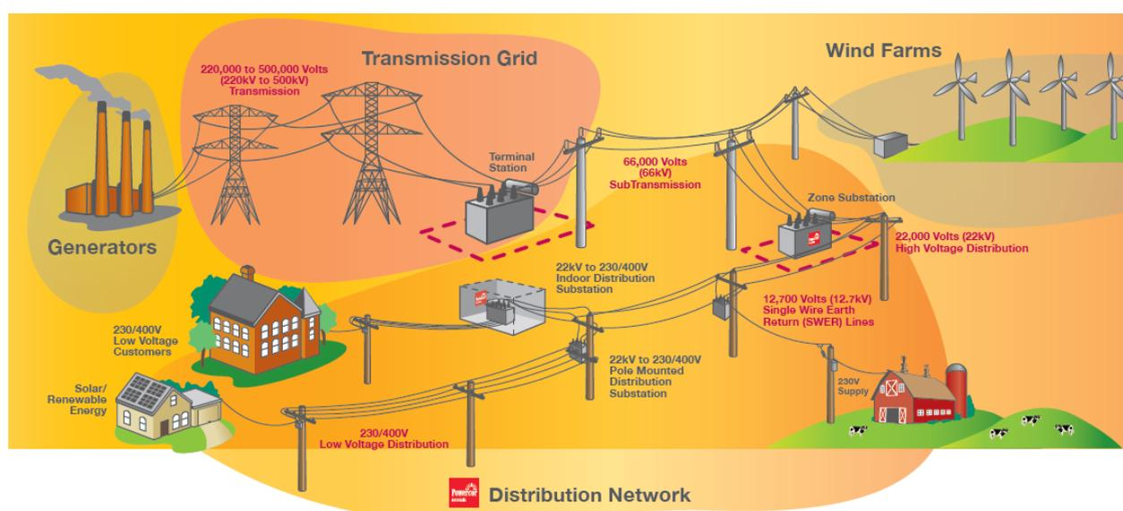
The distribution of electricity is one of four main stages in the supply of electricity to customers. The four main stages are:
