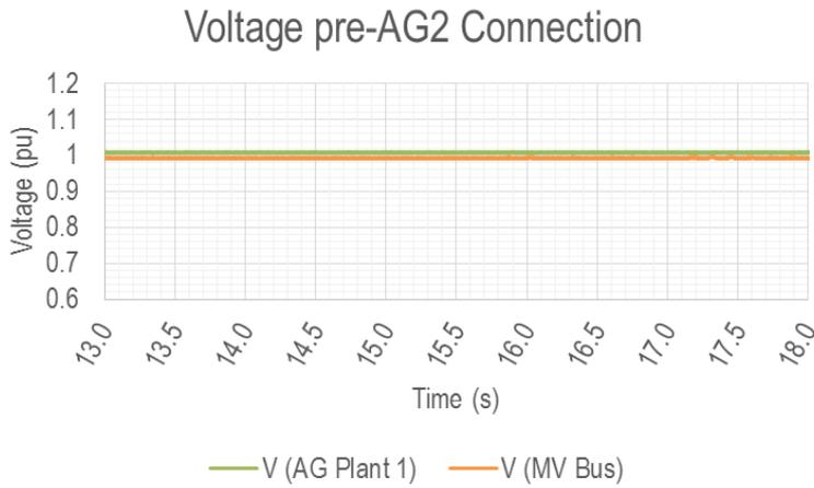
**Figure 8 Dynamic behaviour of sub network pre-AG2 connection**
