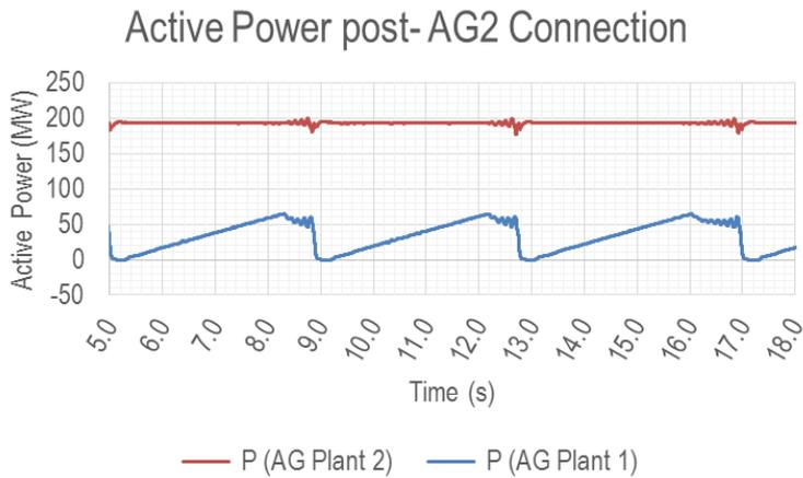
**Figure 12 Dynamic behaviour of sub network post-AG2 connection**
