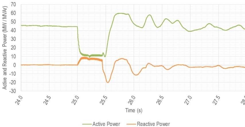
**Both Solar Farm A and B connected – with synchronous condenser at Solar Farm B**
