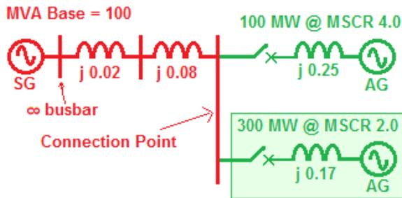
Consider the *connection point* shown in Figure 3 where an existing 100 MW AG is *connected*. A second AG (shaded) wishes to share the *connection point*.
