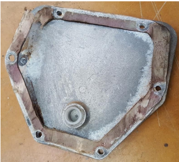
Figure 5 Defect type: internal seal defects
