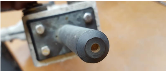
Figure 4 Defect type: vent seal blockages
