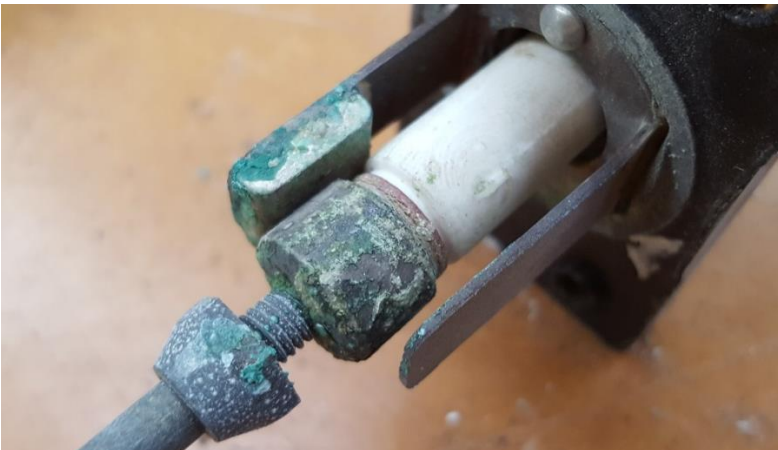
Figure 7 Defect type: damage to contacts
