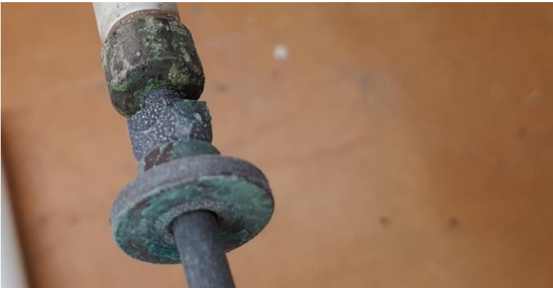
Figure 8 Defect type: poor shaft condition
