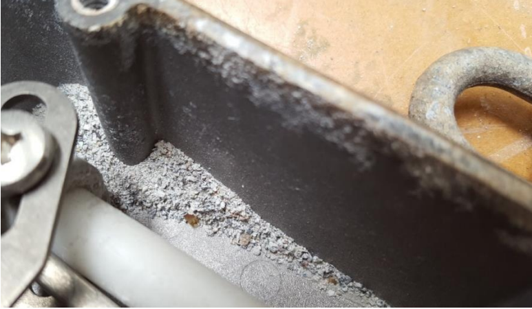
Figure 6 Defect type: aluminium oxidisation
