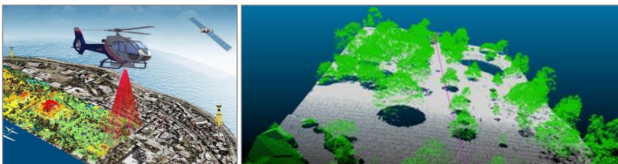
Figure 3.2 Example of LiDAR data visualisation to identify vegetation growth
