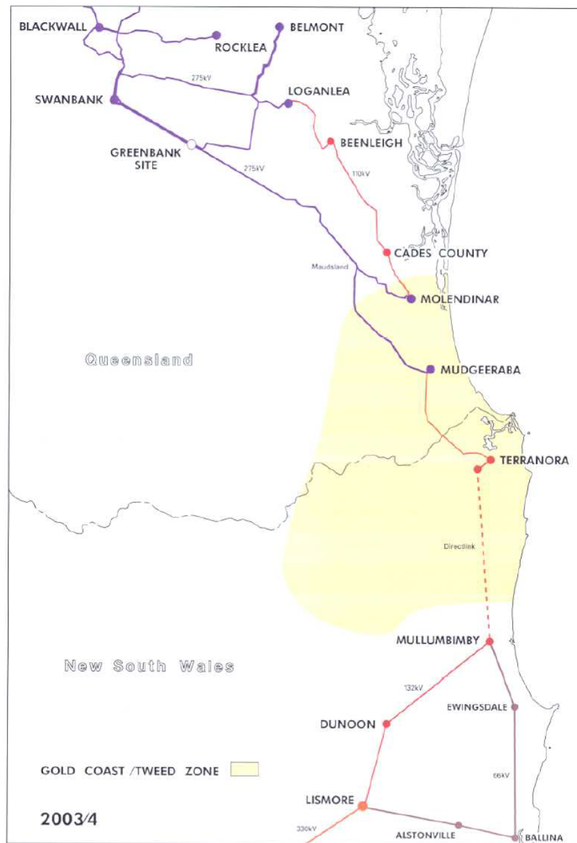
Figure 1: Electricity supply system to Gold Coast/Tweed Area
