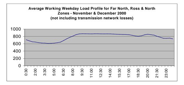
As shown by the graph above, this pattern was in evidence during late 2000. The Townsville gas turbines were required to operate for the majority of the day during the periods that binding grid constraints would otherwise have occurred – an atypical operating mode for peak load generators.
