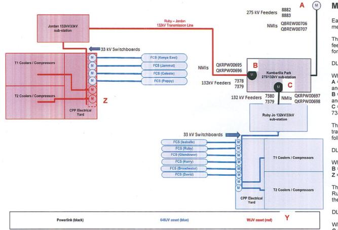
Y = Load measured by the meters at Y
