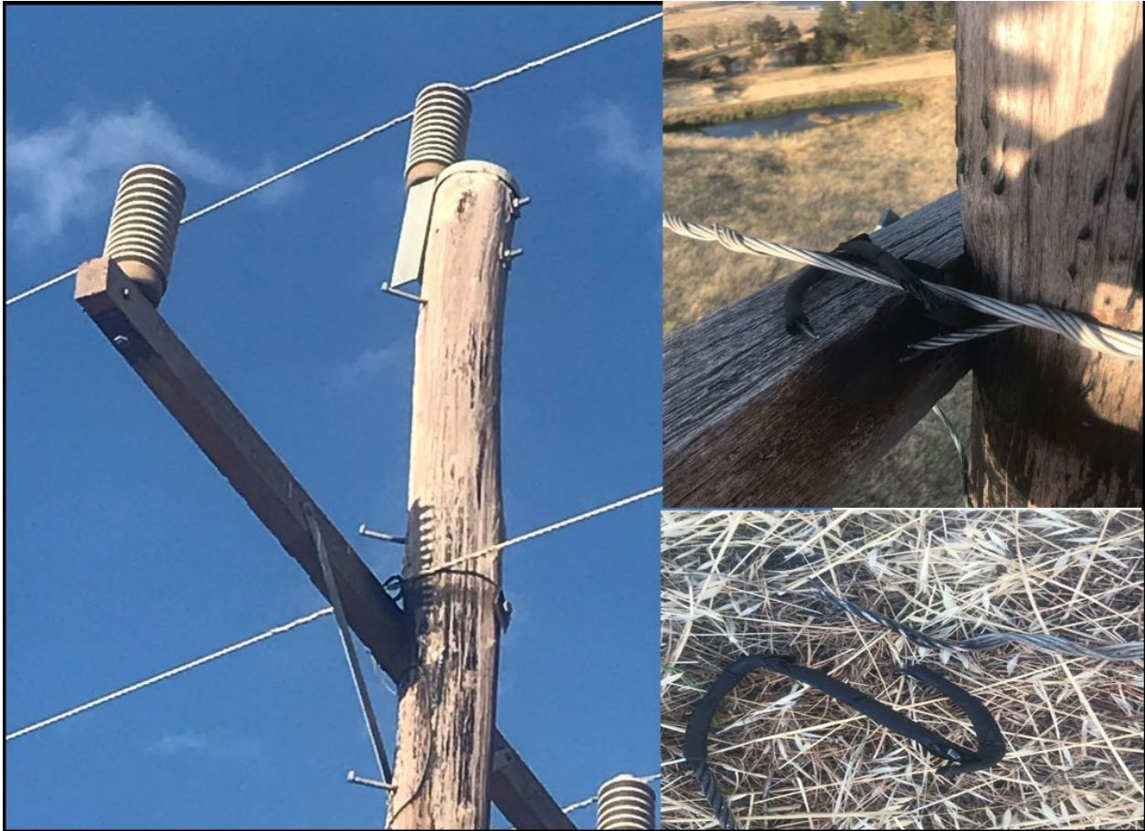
Figure 3 – Cross arm tie failure INCD-2144062-a
