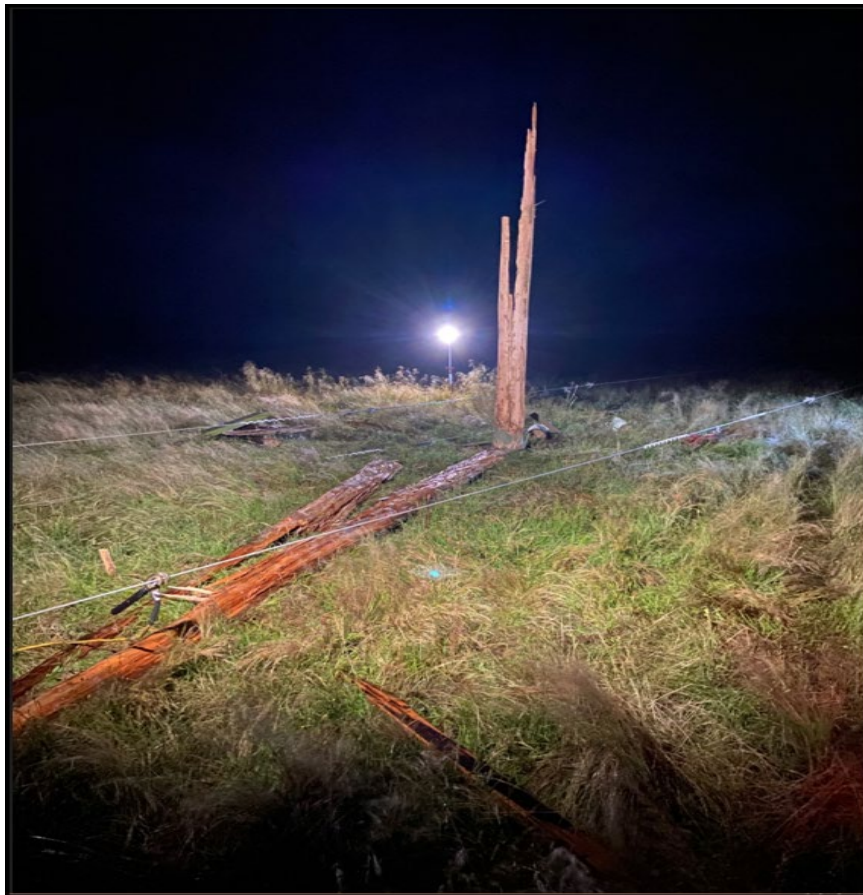
Figure 2 - Timber Pole Failure INCD-97660-q
