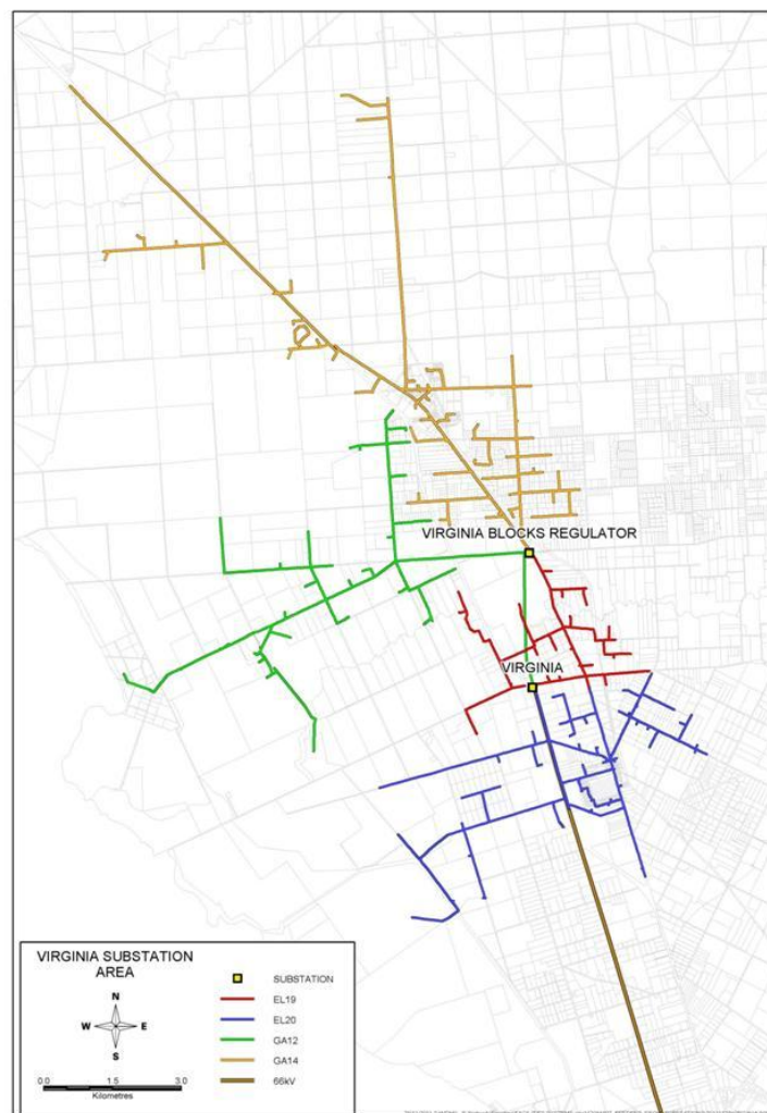
Figure 18: Virginia 66/11kV Zone Substation Supply Area
