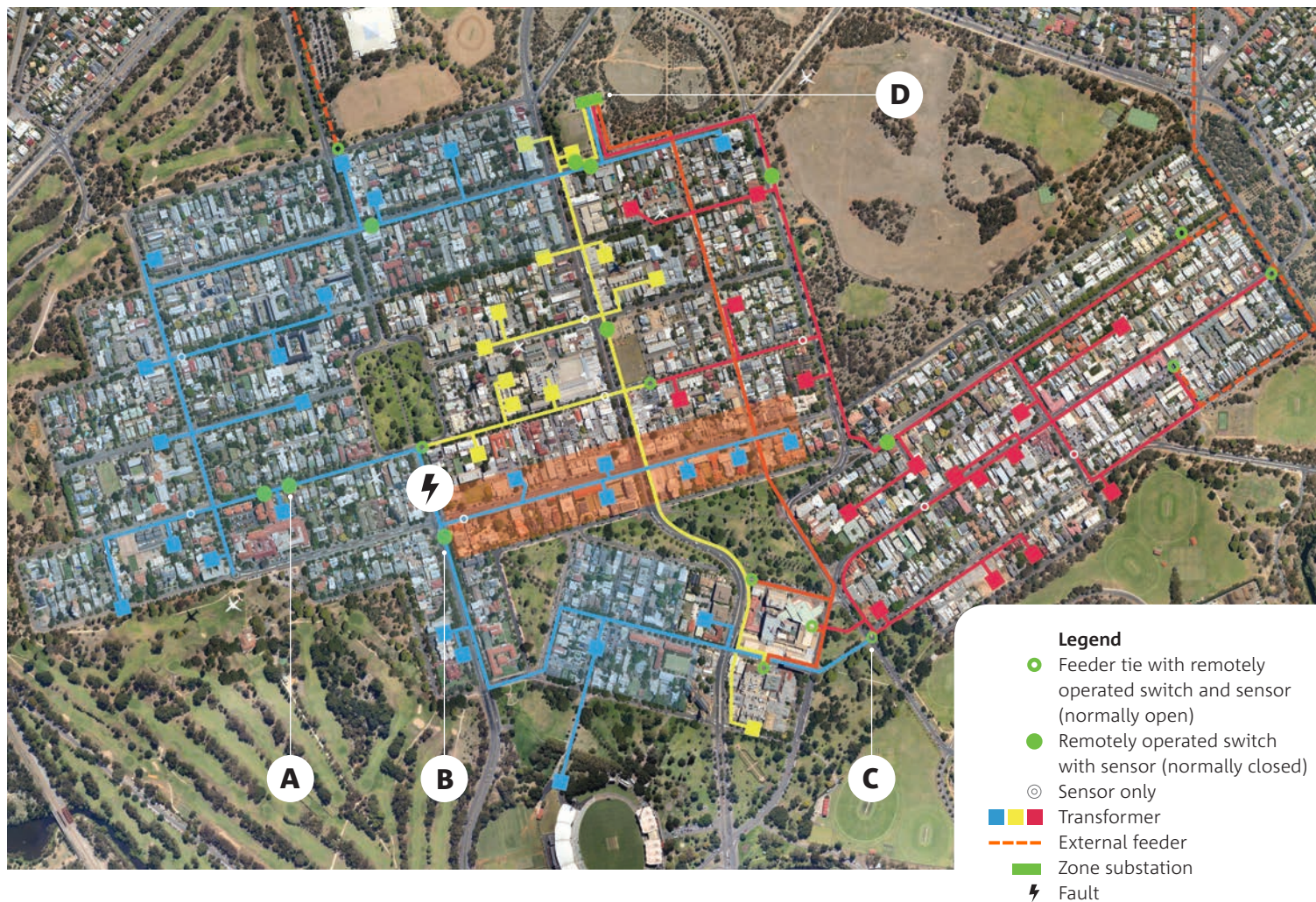
Figure 6.3: In 2028, the urban network will be increasingly interconnected and able to automatically isolate faults, restoring power to the maximum number of customers
