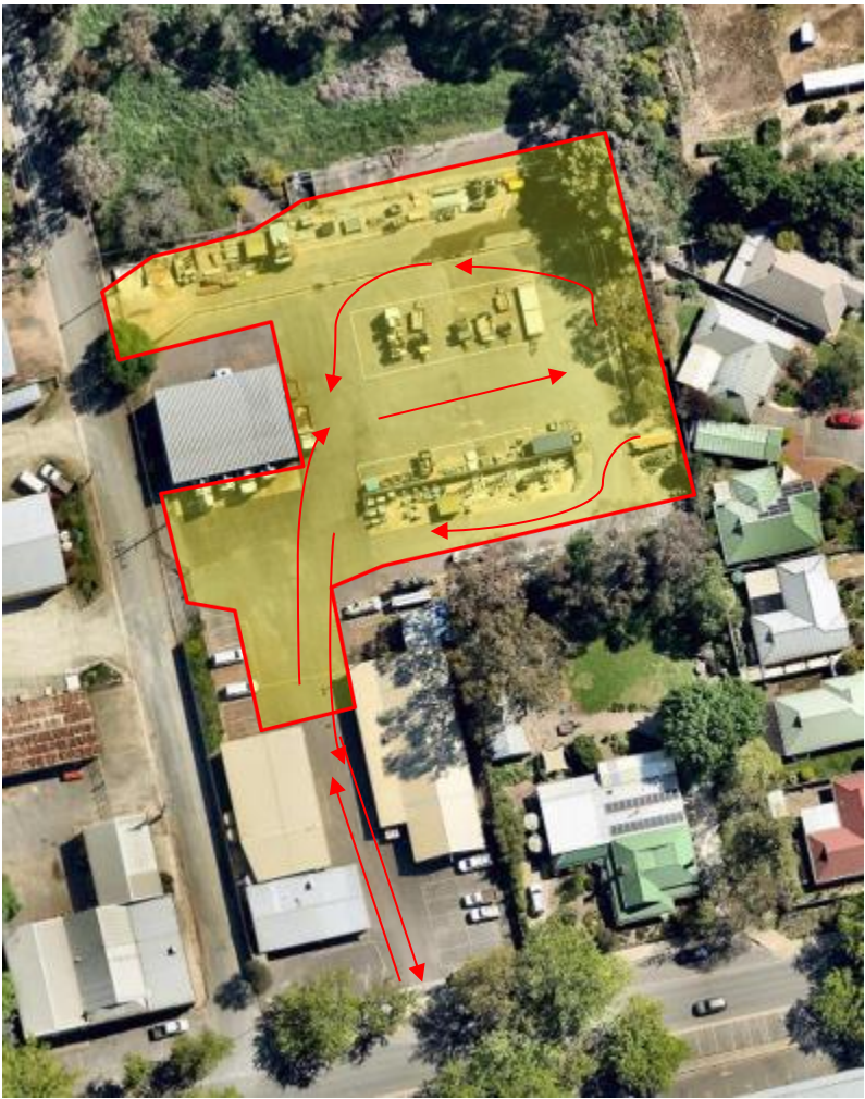
Figure 3 Diagram of poor condition pavement areas and general heavy vehicle flow paths at the site
