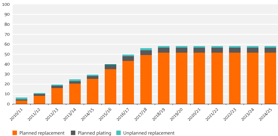
Figure 20.19: Historic and forecast pole replacement and refurbishment expenditure profile (June 2015 $ million)
