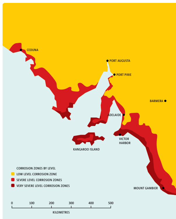
Figure 20.11: Atmospheric corrosion zone map of South Australia
