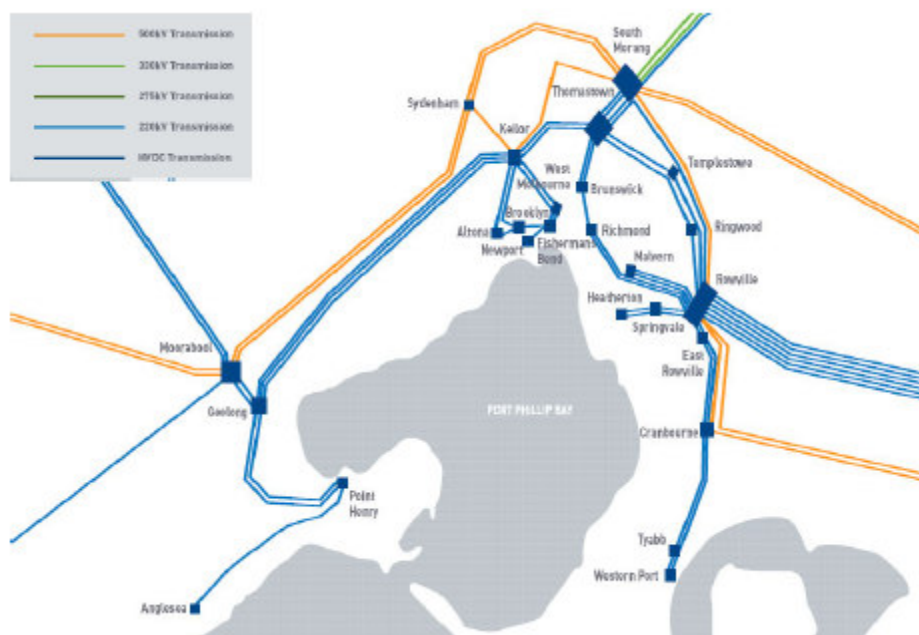
Figure 2.2.2 SP AusNet transmission network – metropolitan Melbourne
