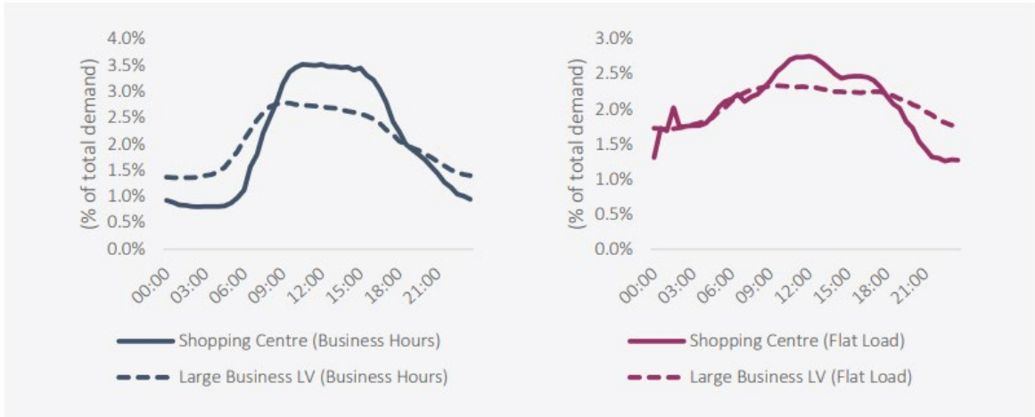
Figure 2 – Load Profiles of Low Voltage Commercial ENs Against Typical Customer Usage Profiles
