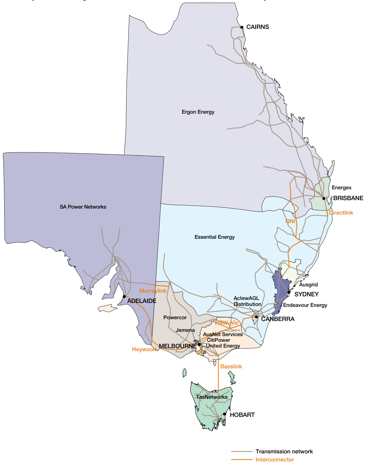
Figure 2.1 Electricity transmission grid and distribution networks in the National Electricity Market
