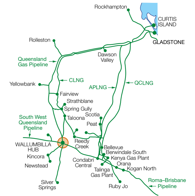
Figure 3.8 Gas pipelines and production facilities near Wallumbilla, Queensland
