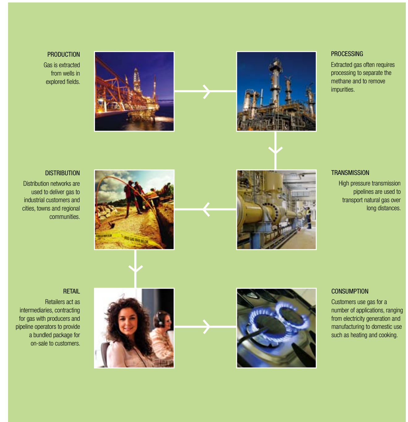
Figure 3.1 Domestic gas supply chain
