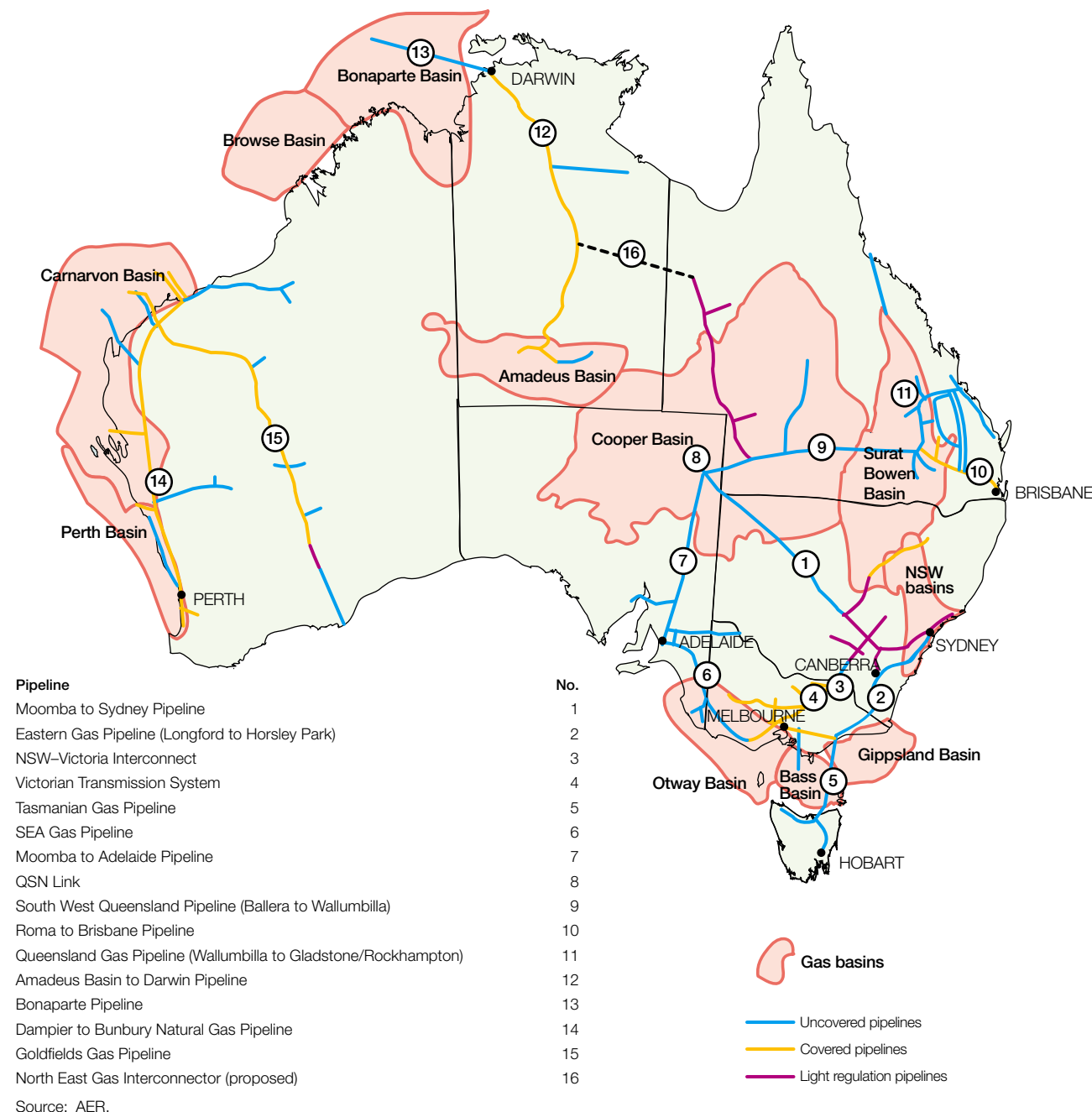
Figure 3.2 Australian gas basins and transmission pipelines
