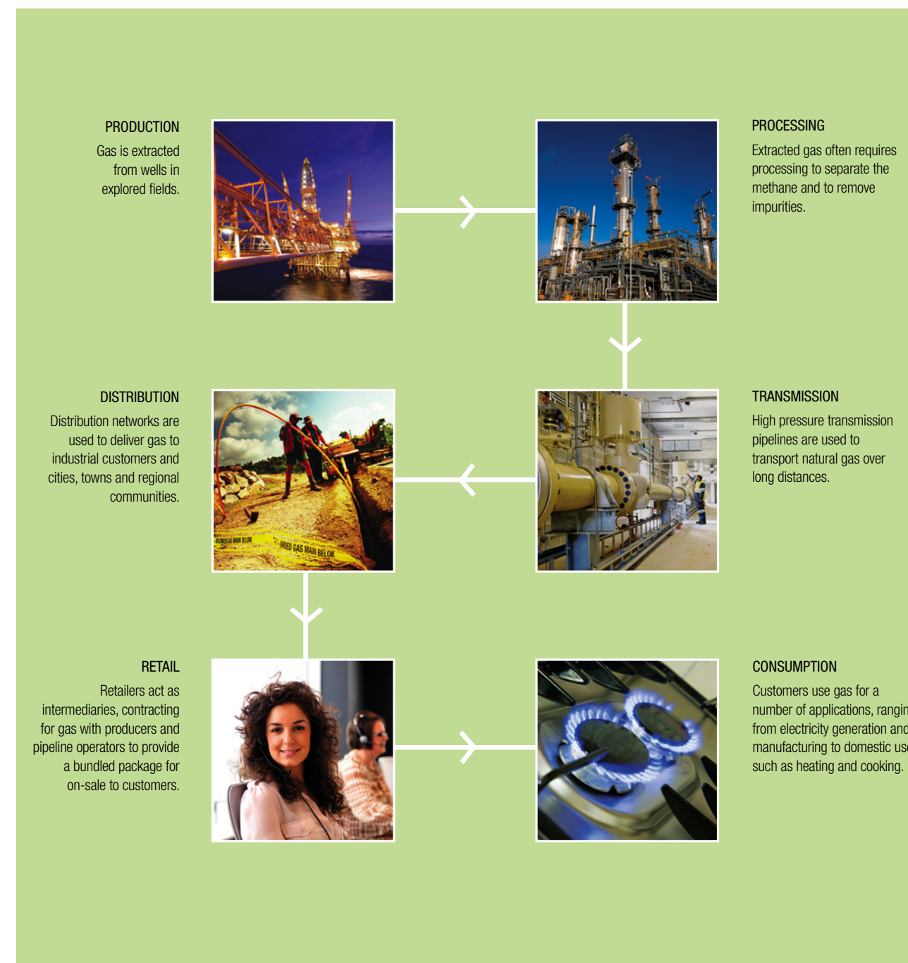
Figure 3.1 Domestic gas supply chain
