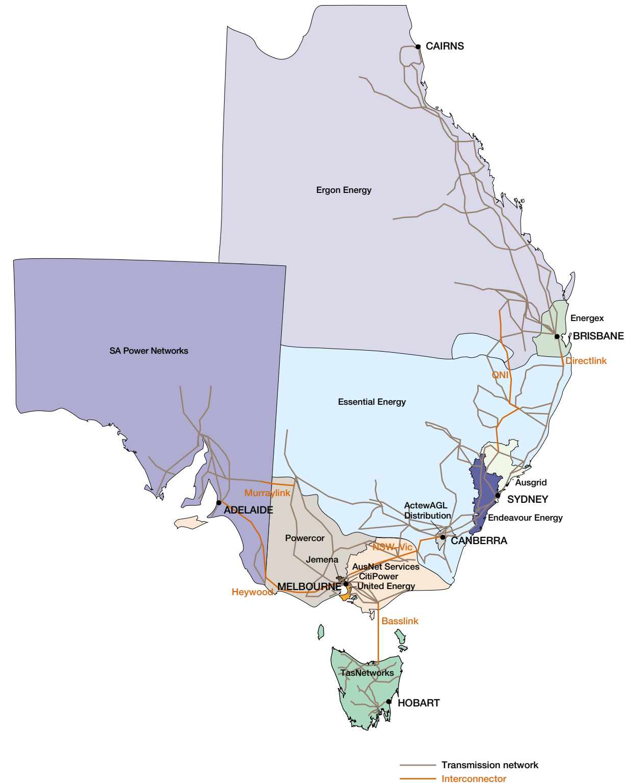
Figure 2.1 Transmission grid and distribution networks in the National Electricity Market
