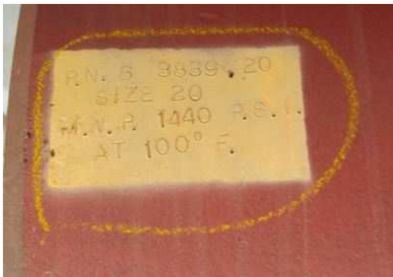
Fig 2.1 Example of Part Number and M.W.P. Stamping.
