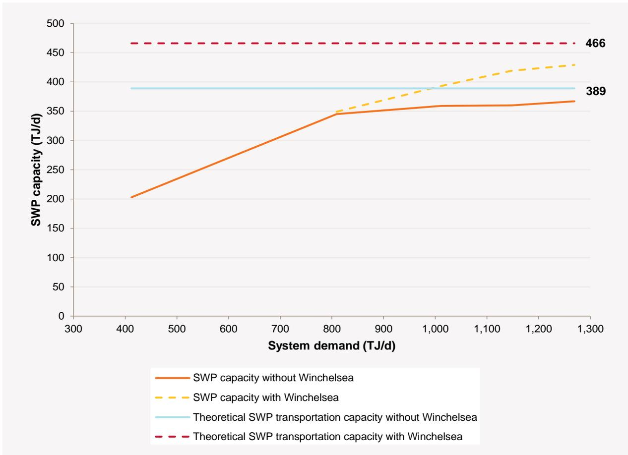
Allowing the SWP to operate at pressures approaching its maximum allowable operating pressure (MAOP) also enables increased injections; however, high pipeline pressures create operational issues for the DTS.
