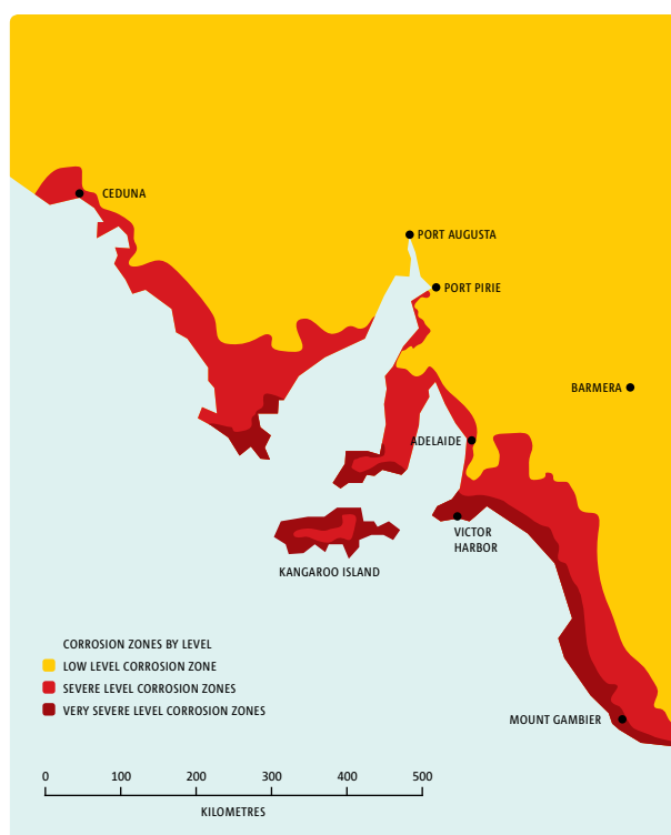
Figure 20.11: Atmospheric corrosion zone map of South Australia
