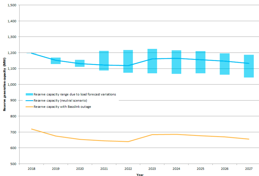
Figure 5-4: Reserve generation capacity variation due to load variations and severe outage
