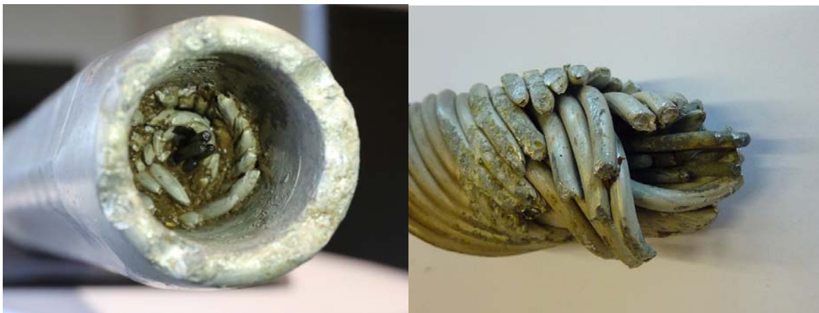
Figure 8: Broken conductor just inside the mid-span joint
