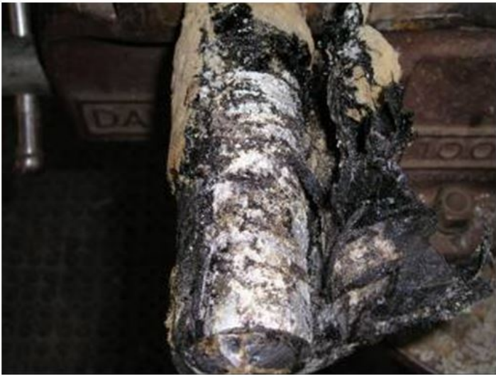
Figure 2 - CONSAC cable failure
