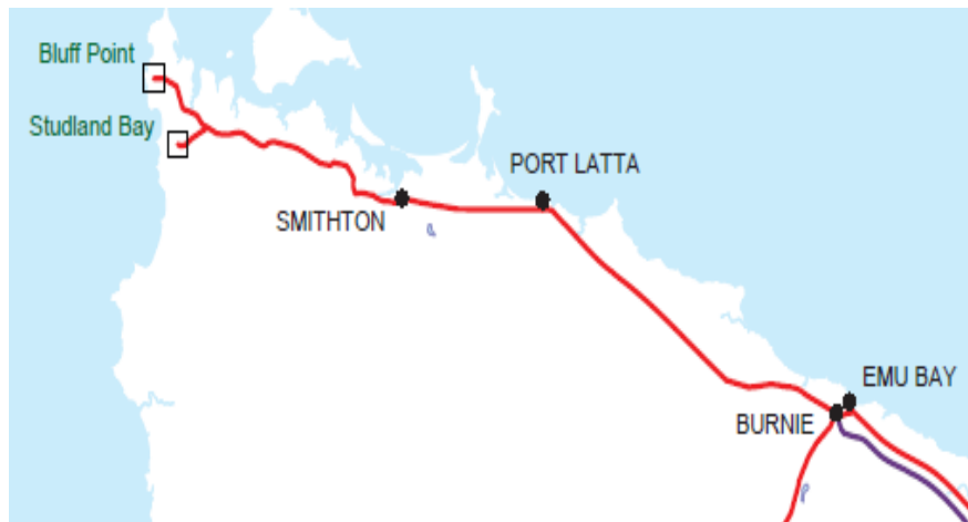
Figure 1: 110 kV transmission network from Smithton to the Bluff point and Studland Bay wind farms
