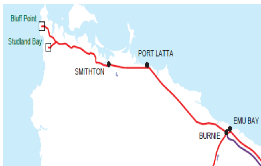
Figure 6 110 kV transmission network from Burnie to the Bluff point and Studland Bay wind farms
