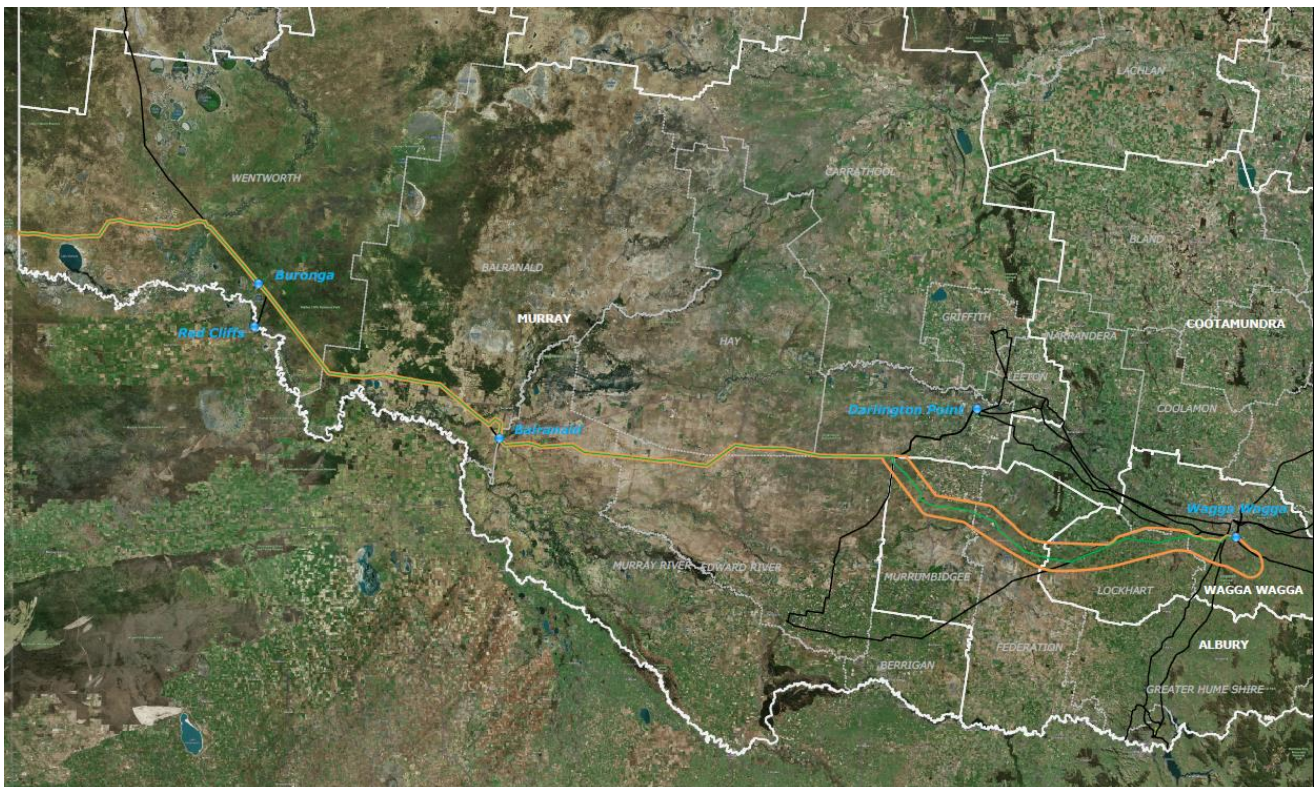
Figure 3.5: Refined PEC line route within NSW
