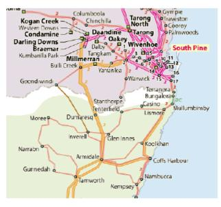
The capacity of the system supplying the Gunnedah, Narrabri and Moree areas is limited by thermal constraints on outage of critical 132 kV lines. These limitations presently exist. Expanded mines in the Gunnedah area have been proposed. Should those proceed, the limitations would be exacerbated.
