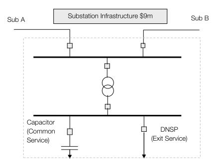
Step 1: The branches are Sub A, Sub B, DNSP, Tie Transformer and PCS.
