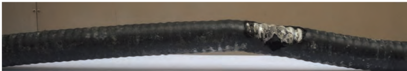
Figure 5: Ausgrid Cable 919 – Failed March 2009
