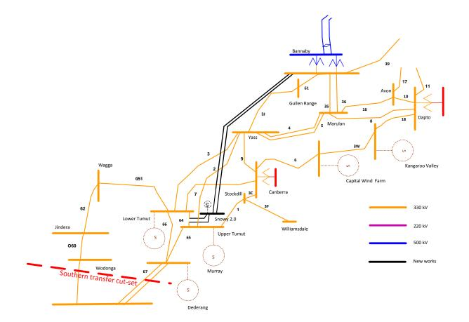
5.6 Option C1: Two single circuit 330 kV transmission lines Tumut – Bannaby (500 kV construction)
