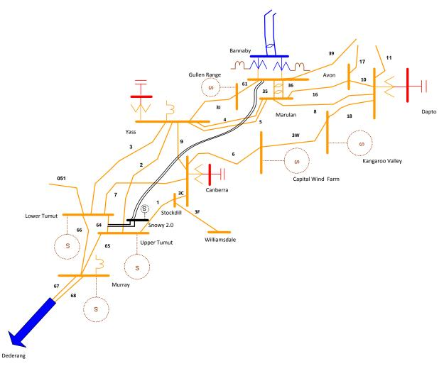
This option involves constructing 2x single circuit 330 kV lines (Invar conductor) from Tumut to Bannaby 330 kV (260km) plus line 64 cut-in loop in/out at Tumut.
