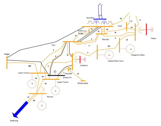
This option involves cutting in to lines O1 (Upper Tumut – Canberra) and 2 (Upper Tumut – Yass) and rebuild as double circuit 330 kV (line O1 – 100 km, line 2 – 147 km), and rebuild line 9 (Canberra – Yass) as double circuit 330 kV (42 km), new double circuit 330 kV from Yass to Bannaby (126 km), and new single circuit 330 kV transmission lines from Snowy 2.0 – Wagga and Wagga – Bannaby.
