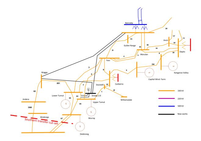
This option involved constructing 3 x single circuit 500 kV (operate at 330 kV) lines (using standard conductors) from Snowy 2.0 to Bannaby, Snowy 2.0 to Wagga and Wagga to Bannaby and line 64 cut-in loop in/out at Snowy 2.0.
