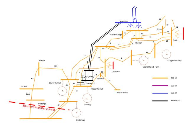
This option consists of constructing 2x single circuit 500 kV lines from Snowy 2.0 to Bannaby (260km), line 64 cutin loop in/out at Snowy 2.0, 3 x 1500 MW 500/330 kV transformers.
