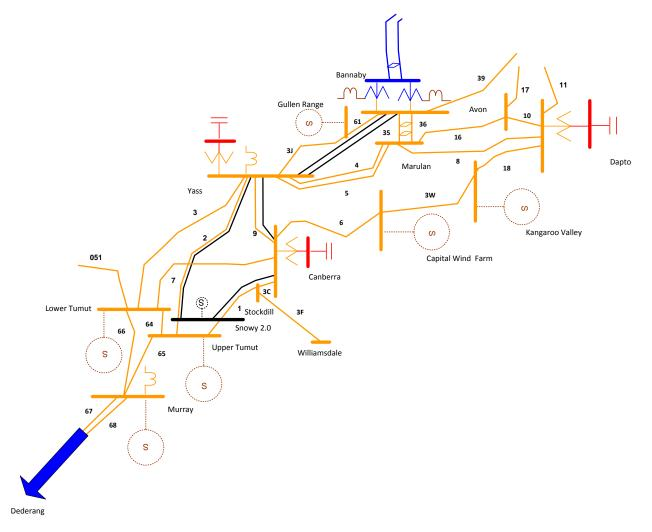
This option involves cutting in to lines O1 (Upper Tumut – Canberra) and 2 (Upper Tumut – Yass) and rebuild as double circuit 330 kV (line O1 – 100 km, line 2 – 147 km), and rebuild line 9 (Canberra – Yass) as double circuit 330 kV (42 km), and new double circuit 330 kV from Yass to Bannaby (126 km).
