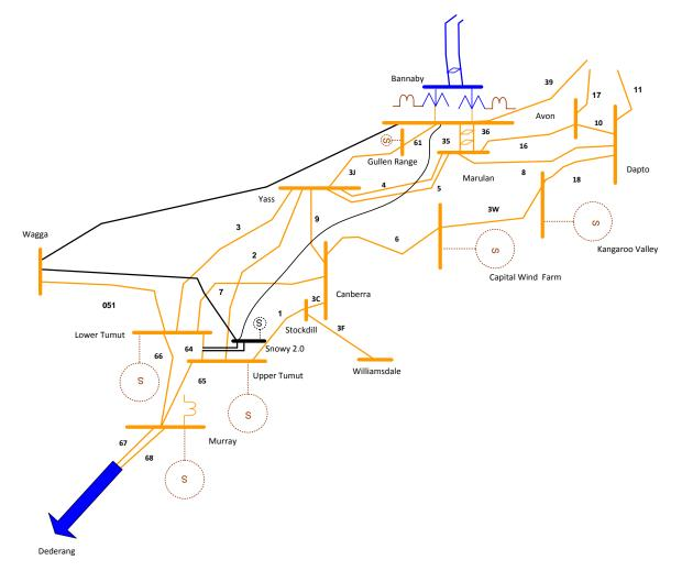
This option involves constructing 3 x single circuit 330 kV lines (Invar conductor) from Snowy 2.0 to Bannaby, Snowy 2.0 to Wagga and Wagga to Bannaby, plus line 64 cut-in loop in/out at Tumut.
