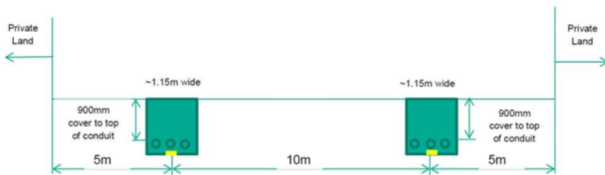
Figure 1 Arrangement of 330kV Double Circuit Underground cable spacing
