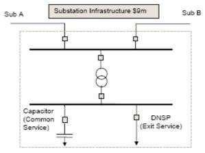
Step 1: The branches are Sub A, Sub B, DNSP, Tie Transformer and PCS.
