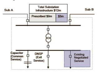
Step 1: The branches are Sub A, Sub B, DNSP, Tie Transformer, PCS and an existing negotiated service.
