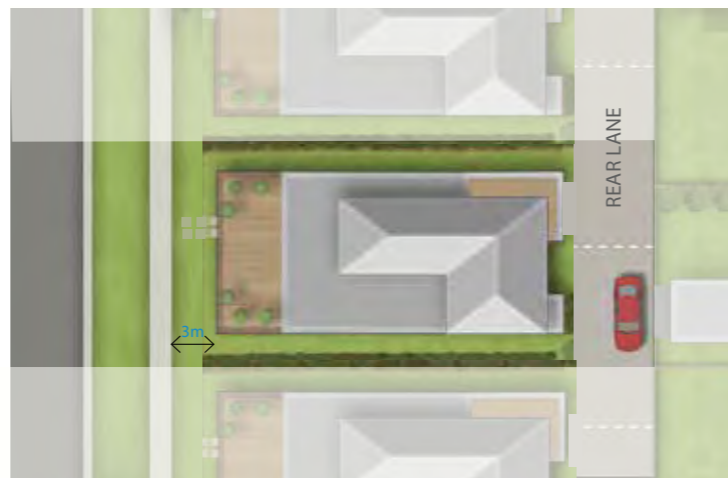
Rearloaded Terraces and Townhouses - garage as part of the main building envelope and balcony private open space.
