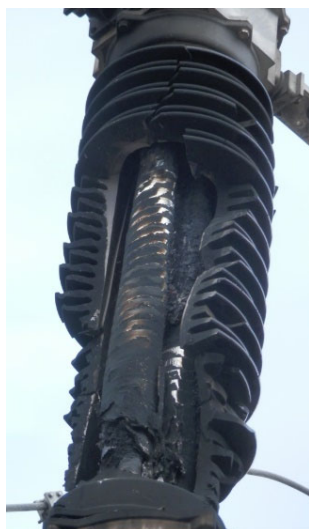
Figure 3| 132kV Current Transformer Explosive Failures
