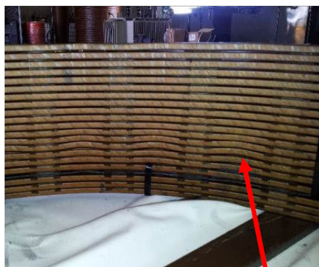
Figure 5| Transformer buckled winding resulting in internal damage then failure
