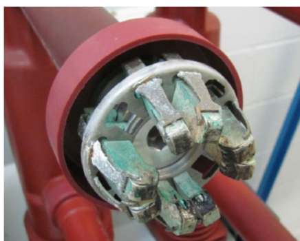
Figure 7| Contact Partial Discharge due to corrosion.
