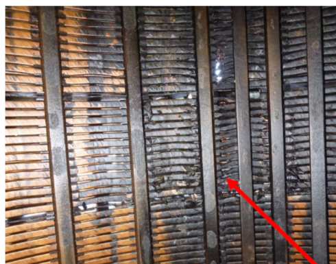
Figure 5| Transformer buckled winding resulting in internal damage then failure
