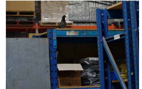
Figure 24: Lack of quick close roller doors creates presence of birds
