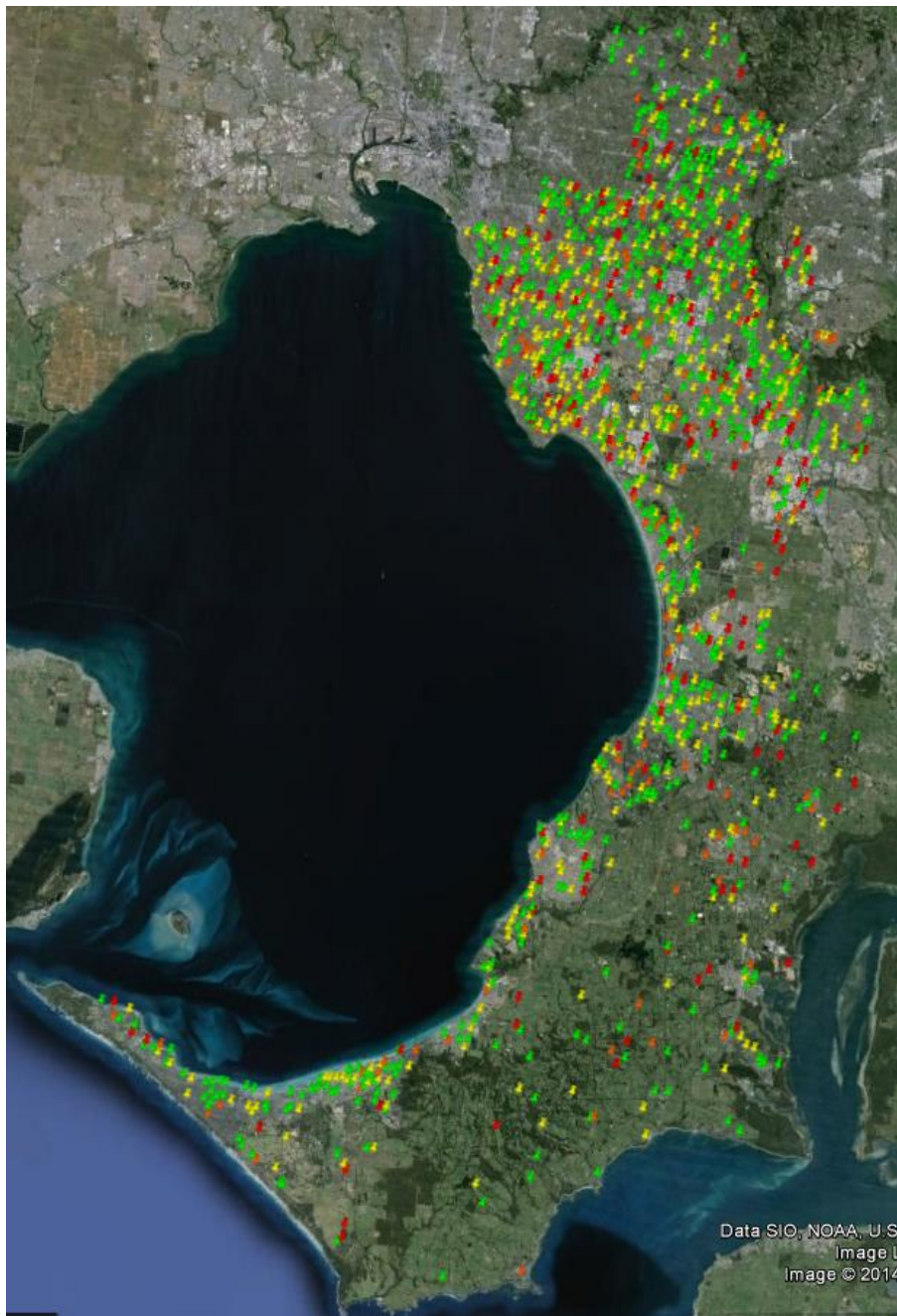
Figure 4-53: Distribution substation spatial utilisation
