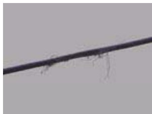
Service rubbed thru by tree
