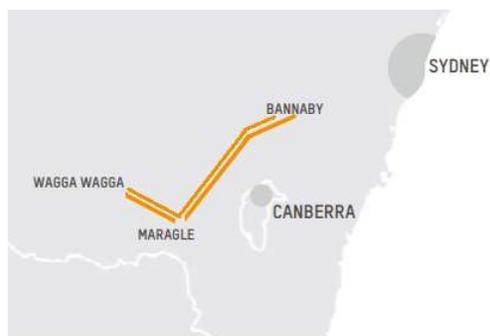
The low-diversity 3C configuration includes routing the Wagga – Bannaby circuit via Maragle. This option has limited diversity potential as all new circuits travel through the same forested areas and parallel existing 330kV circuits in areas of known storm and fire danger using the corridors which have been investigated by the proponent. Although it is not communicated in the PACR, the proponent’s actions to date indicate that this is the favoured option.
