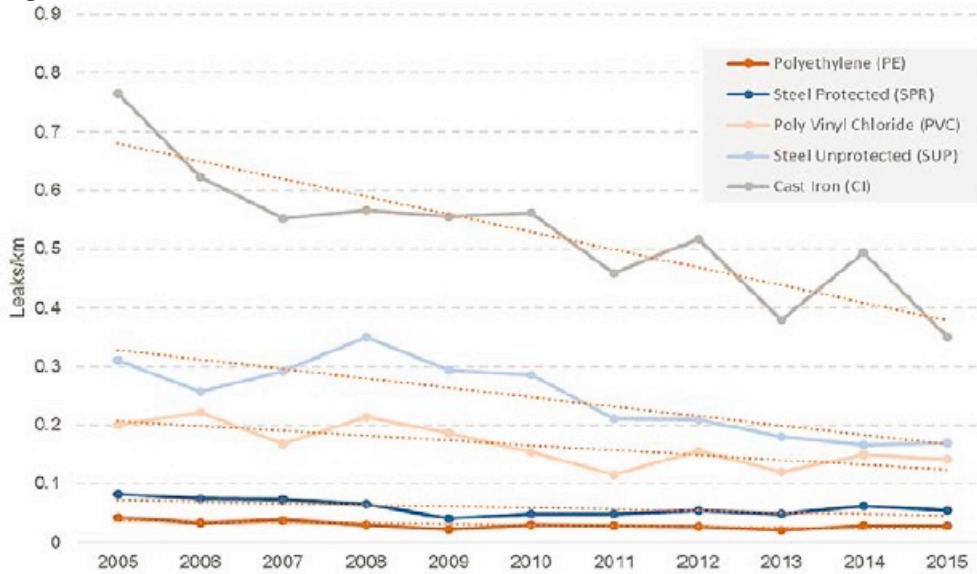
Figure 5: Distribution Mains Leak Incident Rate by Material
